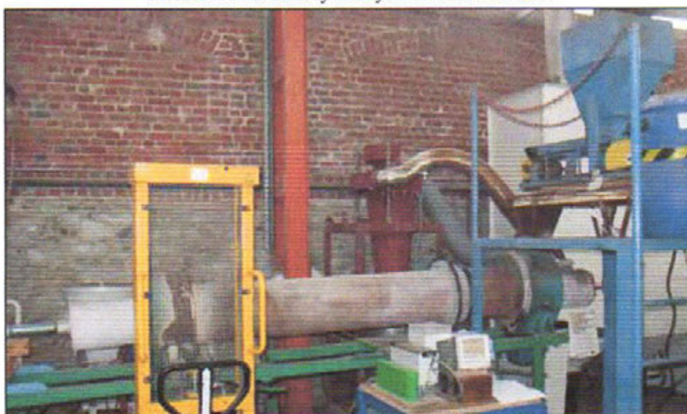
Picture 9 : Laboratory rotary kiln - overall view.
