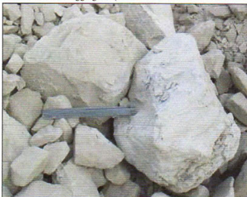
Picture 2 : Coarsest aggregates (size of the reference stick : 200 mm).
