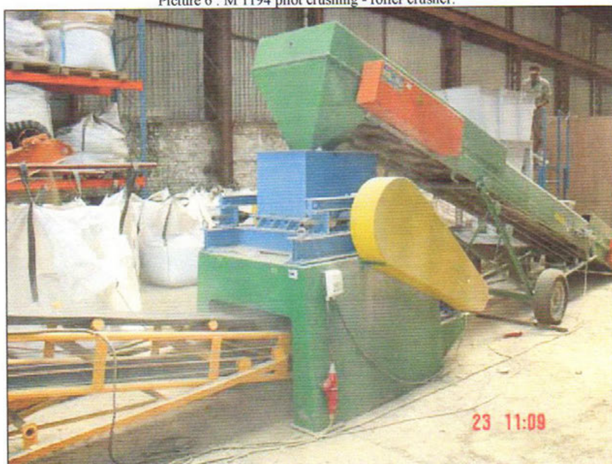
Picture 6 : M 1194 pilot crushing - roller crusher.
